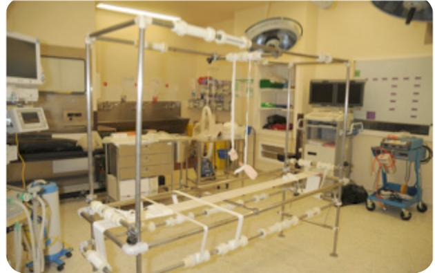
Figure 1. Plaster jacket application frame
